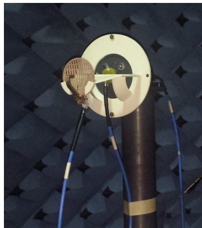
Figure 5-13: Picture of the parabolic reflector antenna inside the anechoic chamber.
