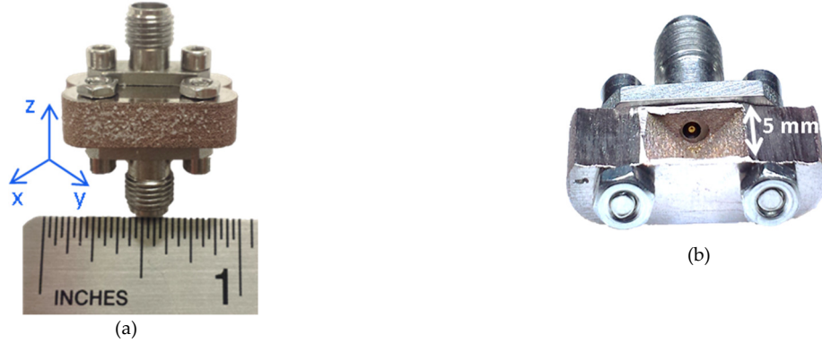
Figure 5-4: 30 GHz cavity resonator. (a) Resonator with connectors. (b) Cross-section of resonator.
